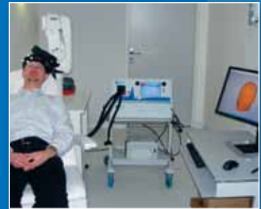
A full and complete Robotized TMS neuromodulation lab (SmartMove which consists a TMS system, Visor Neuronavigation system and the ASA-Lab EEG/ERP system including the Evoke system -VEP and AEP stimulation).
