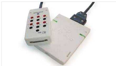
Up to 64 EEG and 6 EMG channels are supported.
